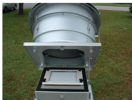
GAS-PM2.5D Series System PM2.5 Inlet Open Position for Access to Filter Paper
