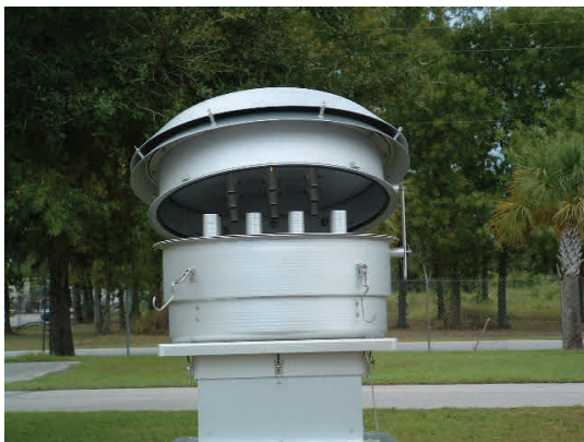
View of PM2.5 Size Selective Inlet illustrating interior features
